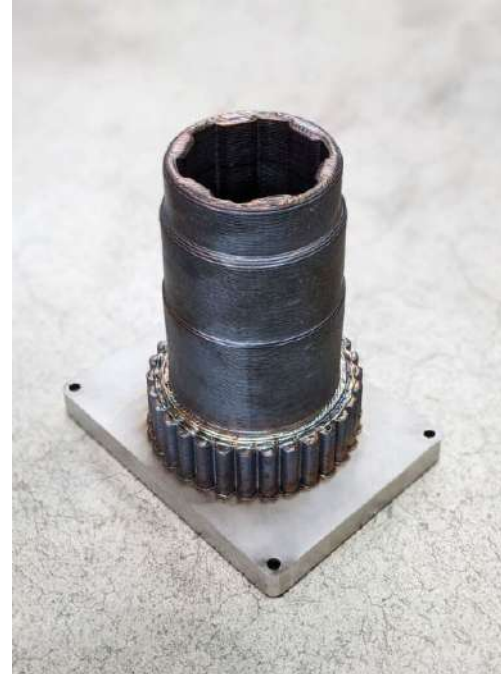
SS308 – Spline Shaft Meltio M450 Size: 132 x 132 x 193 mm Weight: 6,6 kg Print Time: 30 h
