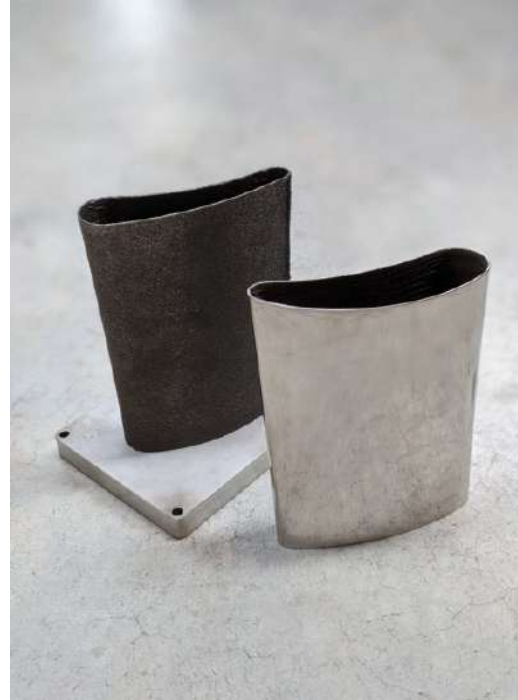
SS316L – Airfoil Cooling Blade Meltio M450 Size: 200 x 152 x 55 mm Weight: 526 g Print Time: 3 h 50 min
