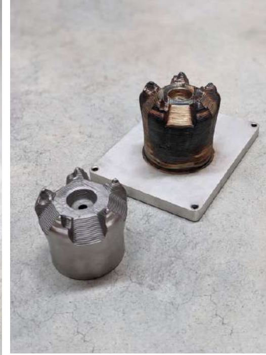
SS316L – Mining Drill Bit Meltio M450 Size: 96,5 x 96,44 x 91,3 mm Weight: 3 kg Print Time: 10 h 5 min
