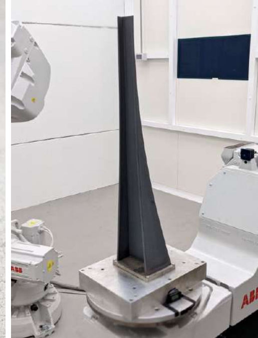
SS316L – Topology Beam Meltio Engine Robot Size: 170 x 130 x 900 mm Weight: 5,95 kg Print Time: 19 h 5 min
