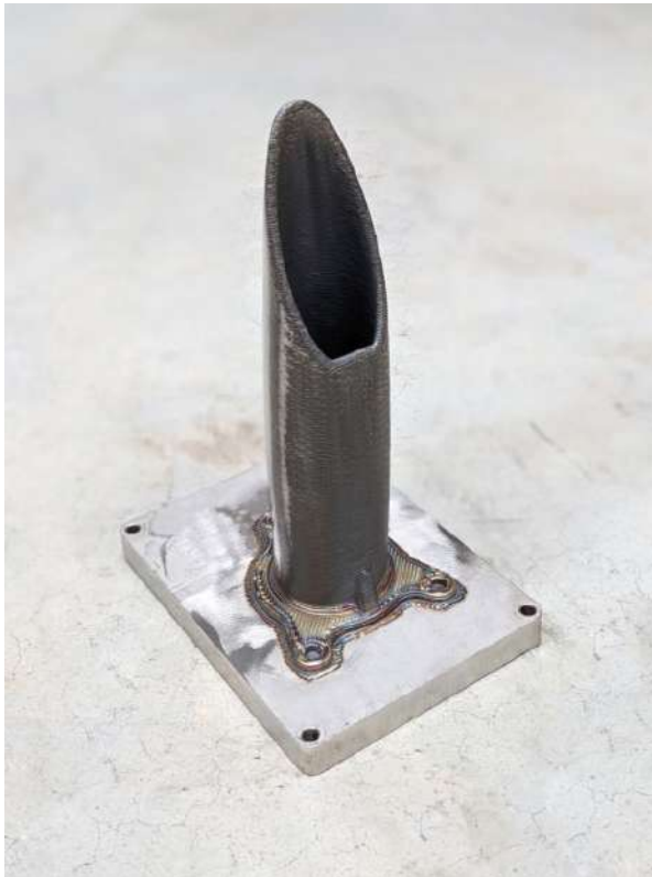
SS316L – Bagging Nozzle Meltio M450 Size: 99 x 116 x 258 mm Weight: 1,78 kg Print Time: 6 h 15 min
