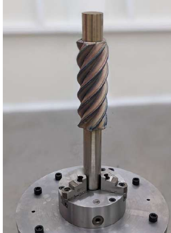
SS316L – Rotary Screw Compressor Meltio Engine Robot Size: 75 x 75 x 230 mm Weight: 2,55 kg Print Time: 7 h 23 min
