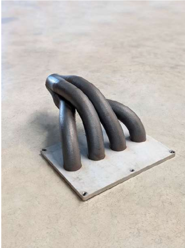
SS316L – Engine Manifold Meltio Engine Robot Size: 205 x 360 x 473 mm Weight: 5,22 kg Print Time: 19 h 23 min
