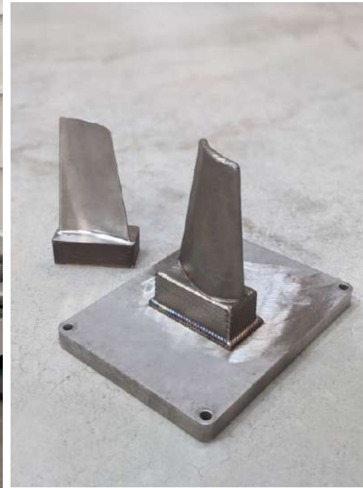
In718 – Gas Turbine Fan Blade Meltio M450 Size: 35 x 75 x 135 mm Weight: 1,11 kg Print Time: 3 h 10 min
