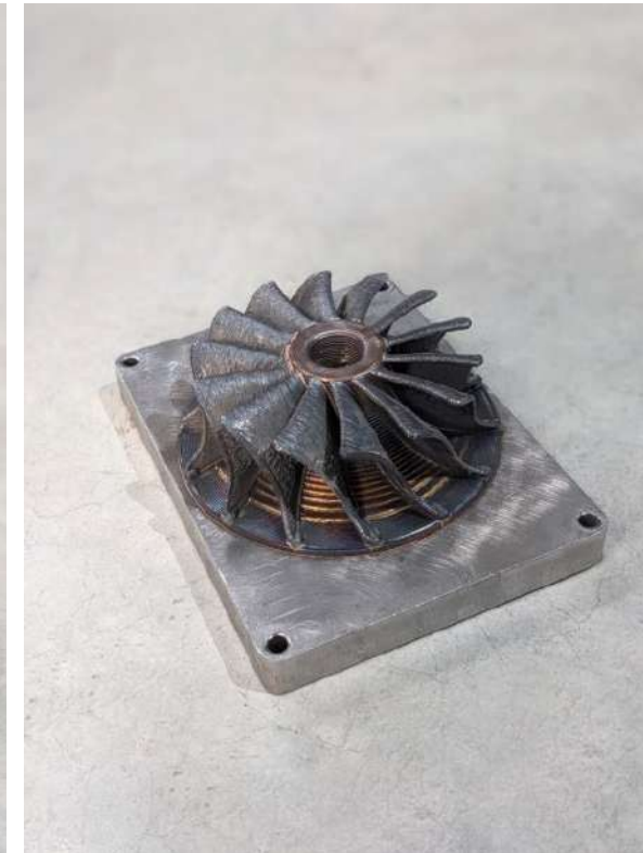
SS316L – Turbo Impeller Meltio Engine Robot Size: 140,3 x 140,3 x 47,7mm Weight: 1,85 kg Print Time: 5 h 48 min
