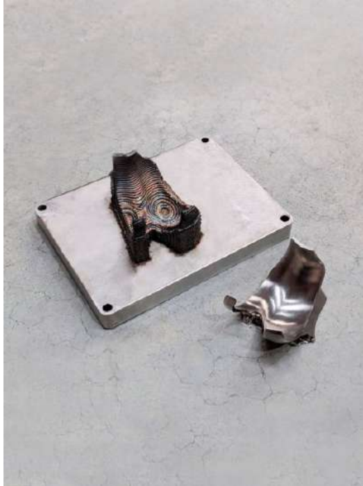
Ti64 – Knee Implant Meltio M450 Size: 99 x 77 x 51 mm Weight: 0,41 kg Print Time: 2 h
