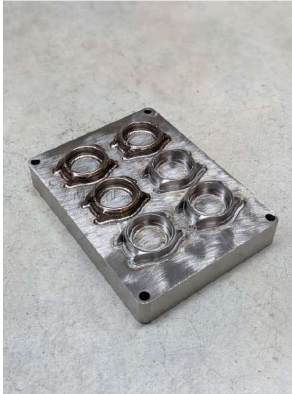
Ti64 – Watch Bezels Meltio M450 Size: 53,37 x 44,59 x 10,85 mm Weight: 29,22 kg Print Time: 5 h 40 min
