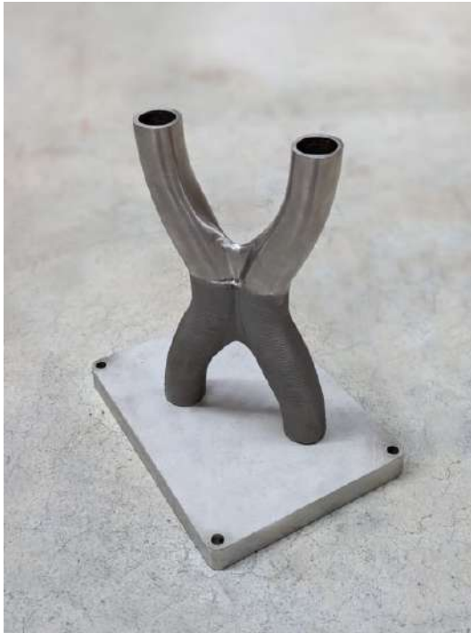
Ti64 – Aircraft Engine Mount Meltio M450 Size: 95,6 x 95,6 x 215,75 mm Weight: 502 g Print Time: 3 h 50 min
