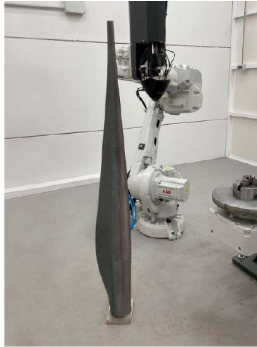
SS316L – Fan Blade Meltio Engine Robot Size: 219 x 133 x 1700 mm Weight: 13,9 kg Print Time: 46 h 34 mi
