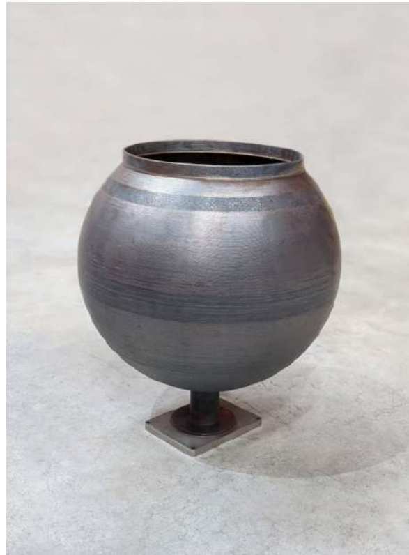
SS316L – Spherical Tank Meltio Engine Robot Size: 500 Ø mm Weight: 29,6 kg Print Time: 81 h 20 min
