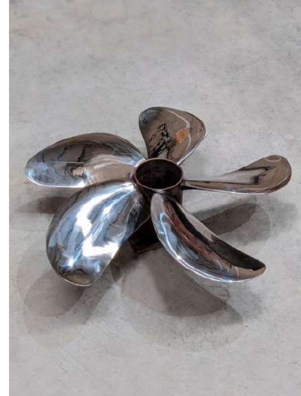
SS316L – Naval Propeller Meltio Engine Robot Size: 600 Ø mm Weight: 12,1 kg Print Time: 43 h 40 min
