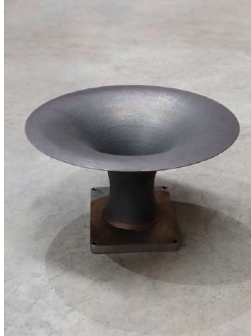
SS316L – Overhang Test Meltio Engine Robot Size: 350Ø mm, H 180 mm Weight: 2,14 kg Print Time: 6 h 26 min
